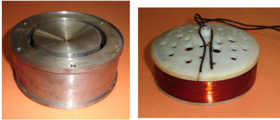
Fig. 3.3. (a) Magnet and iron assembly. (b) Coil former and winding.
