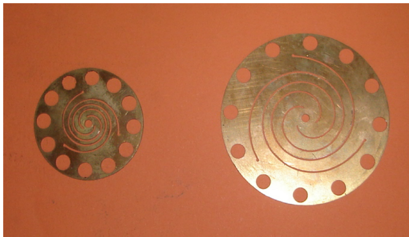
Fig. 3.5. Expander and compressor flexure bearing.
